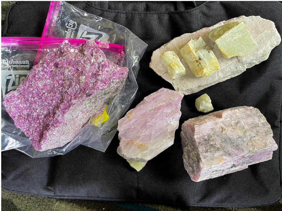
Figure 3: Reconnaissance samples of spodumene and lepidolite from south western Nigeria
