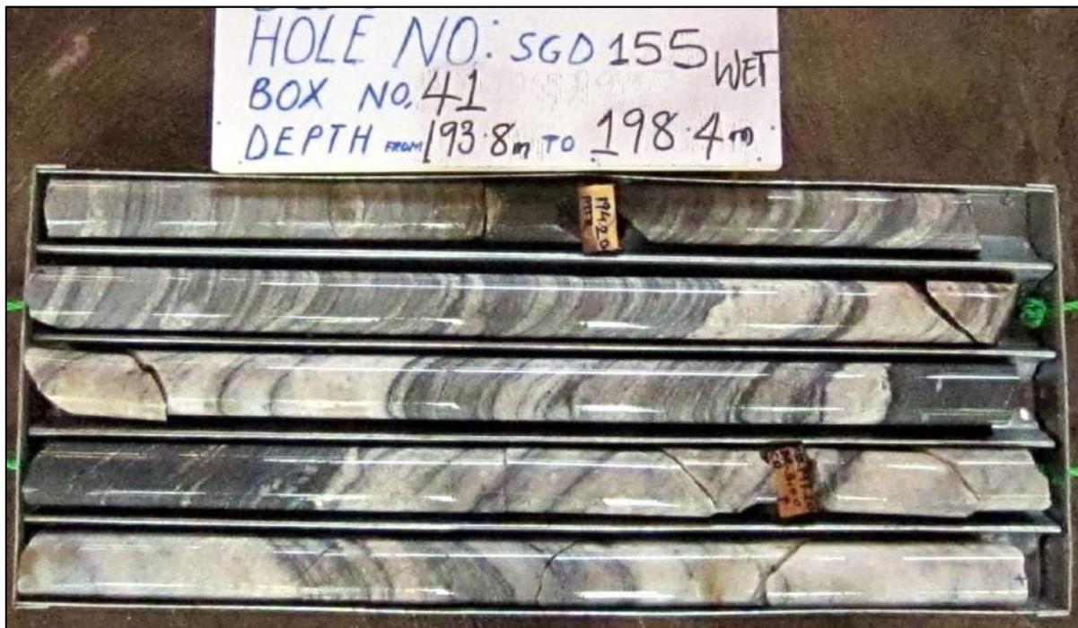
Figure 20 - Intense silica-carbonate alteration of mineralised zone in hole SGD155 (refer to Figure showing detailed log)
