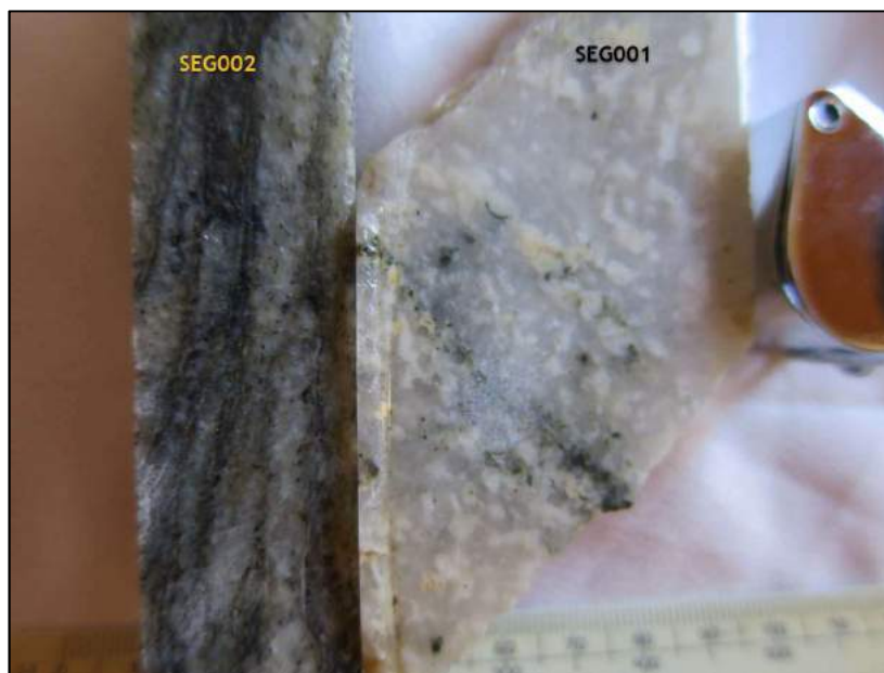
Figure 18 - Pegmatitic quartz-feldspar vein (SEG001) and silicified biotite gneiss (SEG002) from drillhole SHD155
